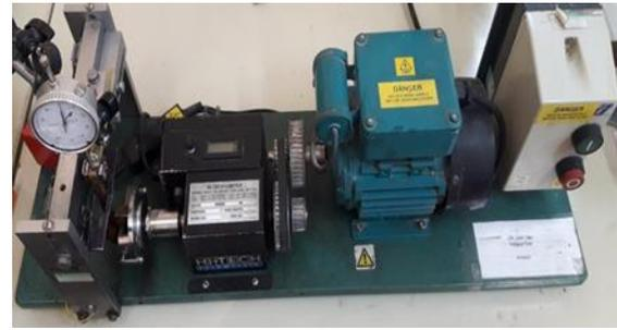
**Fig. 5.** Fatigue test set up: (a) schematic fatigue specimen, (b) alternating bending fatigue testing machine (HSM20).
