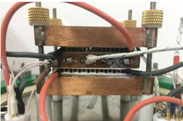
Fig. 3. General view of the measuring cell with installed thermoelectric elements.
