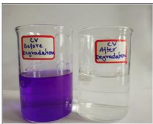
Fig. 27. Results of photodegradation of crystal violet [47].
