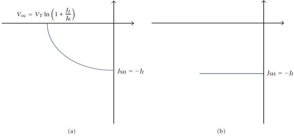
**Fig. 5.**  $J - V$  characteristic of an ideal solar cell with the short- and open-circuit expressions for the axis-intercept points  $V_{oc}$  and  $J_{SH}$ , respectively, (a).  $I - V$  characteristic in the limiting case of a thin-film cell  $l_{n,p} \ll L_D^{n,p}$  (b).
