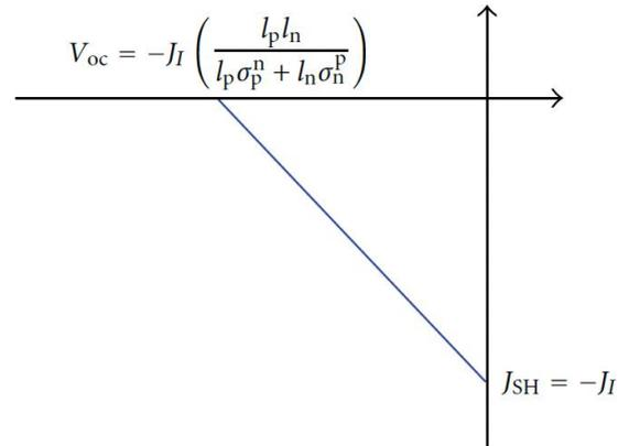
**Fig. 6.**  $J - V$  characteristic of an ideal thin-film solar cell with the new expression for the  $x$  axis-intercept point  $V_{oc}$ .
