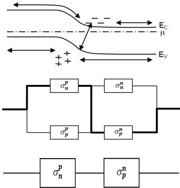
**Fig. 2.** Schematic of the carrier flow in the  $p - n$  junction when volume recombination is strong in the diode ( $\tau_{n,p} \rightarrow 0$ ). For strong recombination, both electron and hole flows are strongly coupled at the diode junction.
