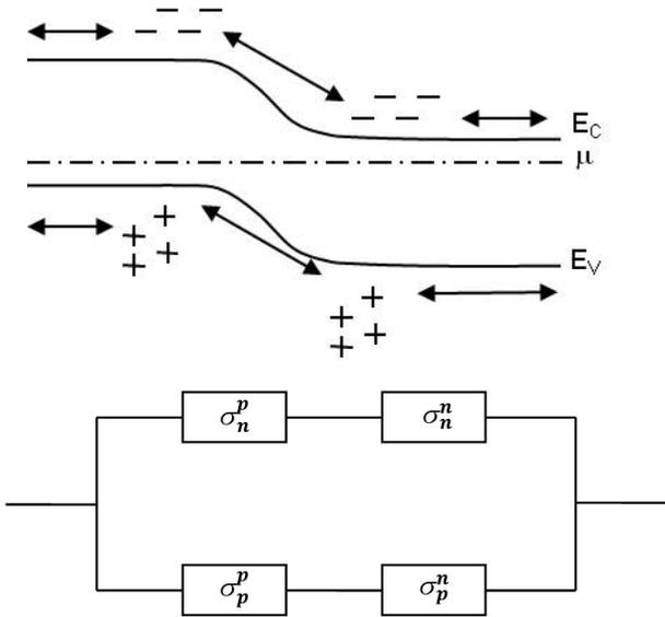
**Fig. 1.** Schematic of the carrier flow in the  $p - n$  junction when volume recombination is weak in the diode ( $\tau_{n,p} \rightarrow \infty$ ).  $E_C$  and  $E_V$  are the conduction and the valence band-edges respectively. Electron and hole flows are mutually uncoupled and independently contribute to the current at the device terminals.
