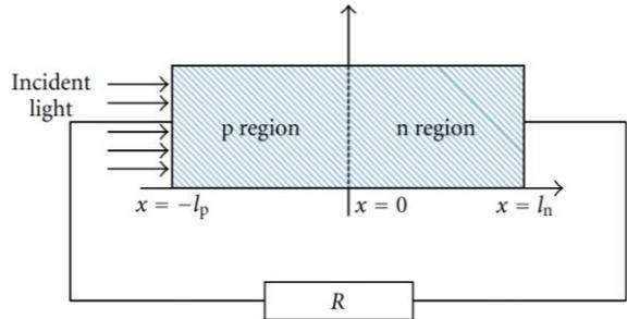
**Fig. 4.** Solar cell diode with an external resistor load.
