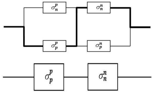
**Fig. 3.** Schematic of the carrier flow in the  $p - n$  junction when volume recombination is very strong.
