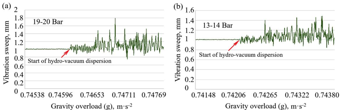
**Fig. 5.** Vibration of the dispersion chamber of the hydro-vacuum machine before and after the working process. (a) Vibration's sweep, mm and overload dynamics before optimization of operating parameters and water pressure, (b) after optimization (Aluminum, dispersion temperature 740°C).
