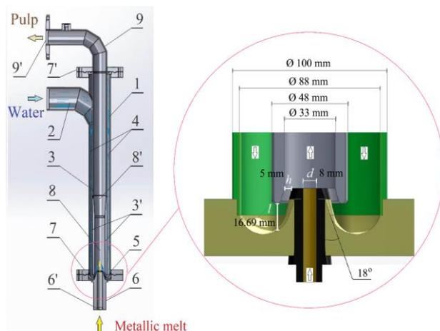
**Fig. 1.** The main technological unit of the device for hydro-vacuum dispersion of melts.
