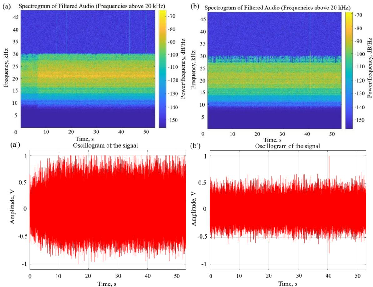
**Fig. 7.** Acoustic spectrum of the hydro-vacuum dispersion process of aluminum in the established operating mode of the equipment: (a, a') before optimization and (b, b') after it.
