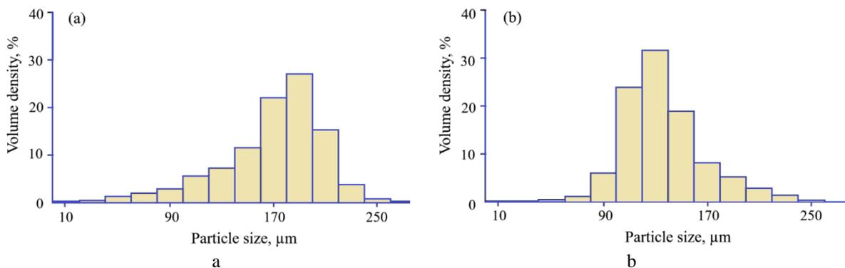
**Fig. 9.** Granulometric composition of obtained powders before (a) and after (b) optimization of the hydro-vacuum dispersion process.
