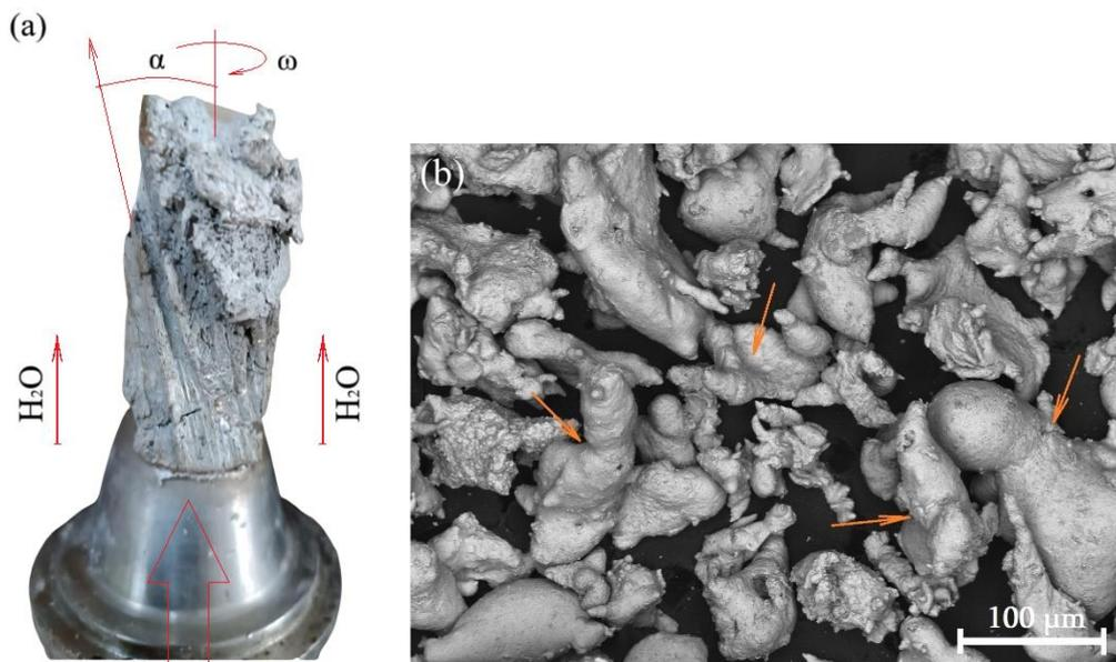
**Fig. 8.** (a) Effect of hydromechanical impact on the flow stream of the sucked metal, and (b) powdery particles obtained as a result of dispersion, fraction 10-100  $\mu\text{m}$ .
