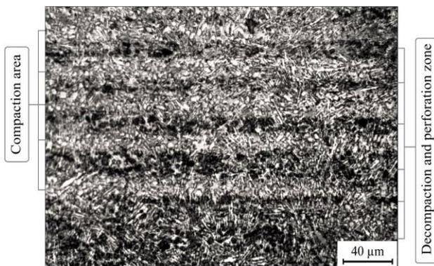
**Fig. 3.** Microstructural segregation, gradient migration and non-equilibrium stress in duralumin powder particles dispersed by hydro-vacuum method.
