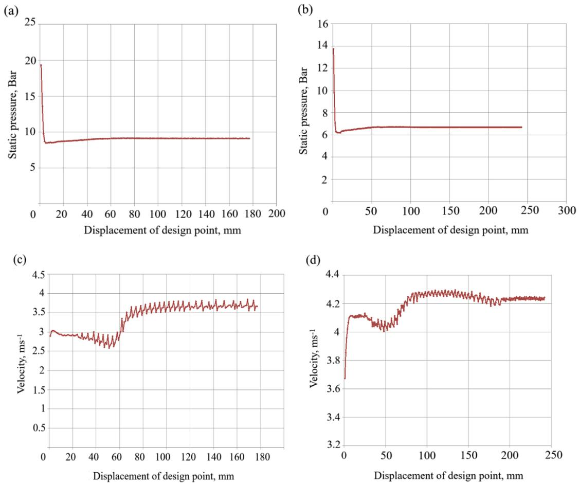
**Fig. 4.** Results of the simulation study: indicators of pressure drop and velocity increase of the water supplied to the dispersion chamber in relation to its vertical location, before optimization ((a), (c)) and after optimization ((b), (d)) of the dispersing process.
