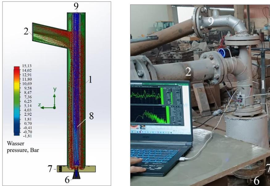
**Fig. 2.** A graphical simulation model of the hydro-vacuum dispersion process and experimental research prototype in semi-industrial conditions.
