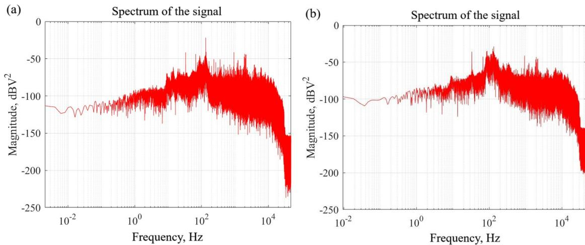
**Fig. 6.** Amplitude spectrum of the audio signal before and after pumping the melt into the dispersion chamber: (a) spectrum before optimizing the geometrical parameters of the converging duct (5); (b) after optimizing.
