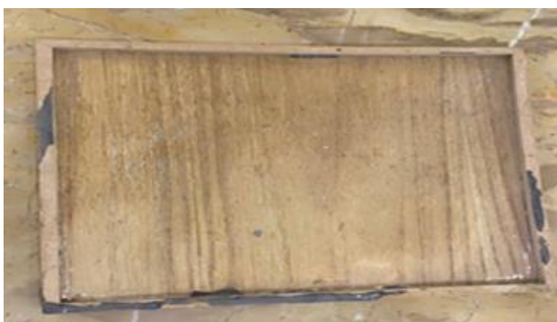
Fig. 2. A wooden mold for free vibration composite FGMS sample (300 x 300 x 10 mm).
