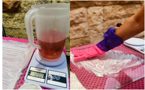
Fig. 5. The hand lay-up technique used for fabricating composite FGM samples.
