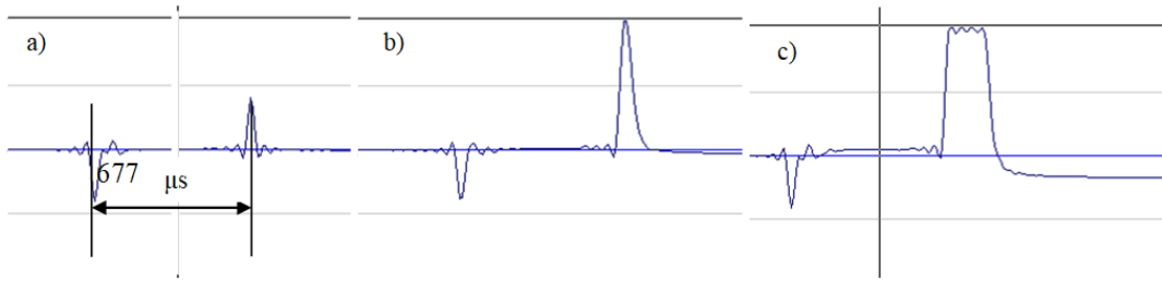
Fig. 4. The photodiode FD-7K records the plasma flash during the gallium arsenide irradiation process at different laser pulse intensities: 16 MW/cm 2 (a), 25 MW/cm 2 (b), 40 MW/cm 2 (c).
