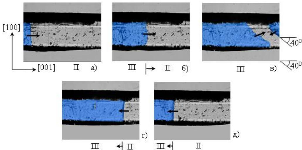
**Fig. 3.** Optical micrographs illustrating the formation and growth of III and II modifications of crystals during the repeated transformation of  $II \leftrightarrow III$  in a  $K_{0.940}Cs_{0.060}NO_3$  single crystal (magnification  $\times 90$  times). a, b, c – growth of the embryos of III – modifications inside the II - crystal; d, e – reverse  $III \rightarrow II$  transformations.
