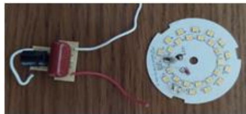
Fig. 7. Light bulb with 28 light diodes. Electronic driver. on the limiting capacitor.
