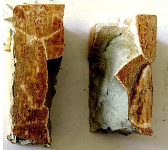
Fig. 3. Typical formation of amorphous mass on the research formulations based on PCT I-100.
