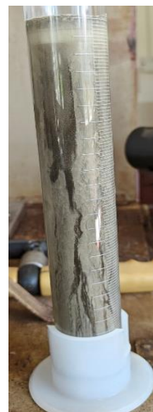
b) sedimentation channels in water separation
