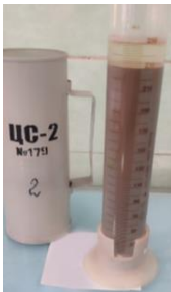
a) water separation of the plugging mud
